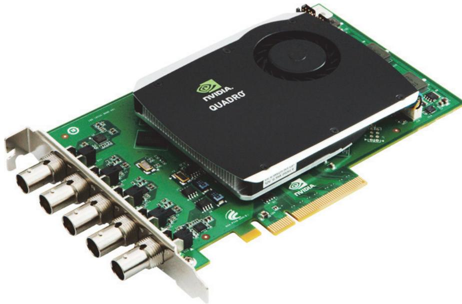
Currently the NVIDIA Quadro SDI Capture card can only be used with the NVIDIA SDI option. Vizrt's application of this card is mainly in time critical environments like virtual studios and sports applications as it has a stable latency from input to output (of 4 frames).
