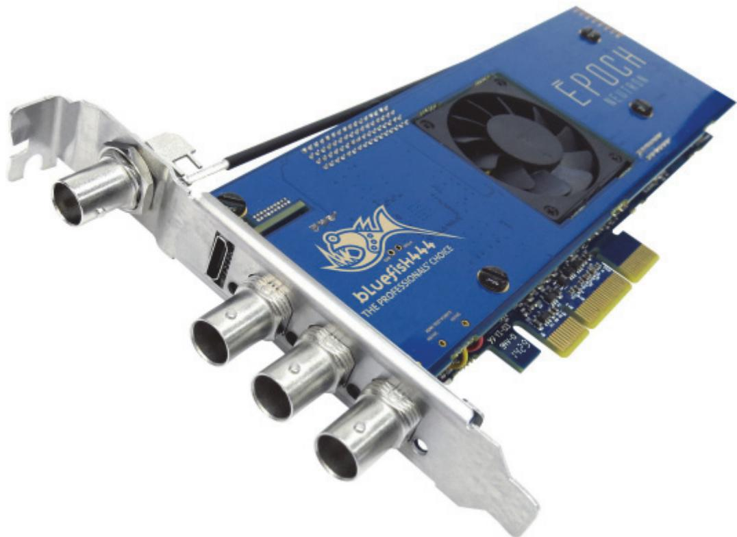
The Epoch | Neutron is a full-length PCIe card with three bi-directional multi-format I/O BNC connectors that support dual link configurations. For use with Viz Engine, the card needs to be configured with one input and one output. Of the three BNC connectors, the first two do SD, HD, 1.5G, ASI, AES and LTC as either input or output. The third is used for GenLock.
