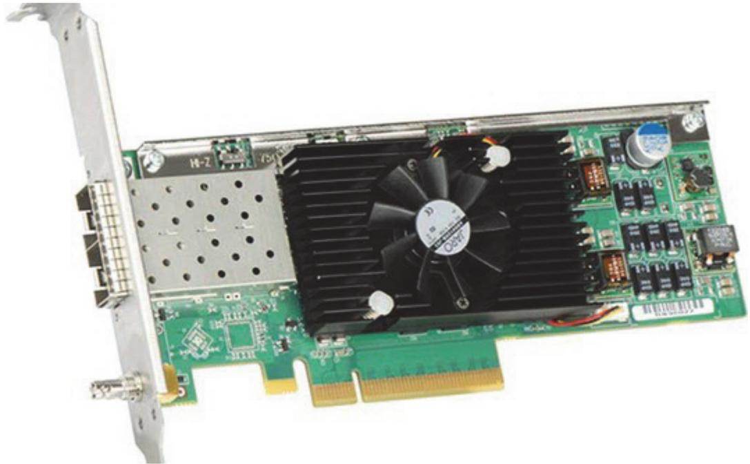
The card contains two enhanced small form-factor pluggable (SFP+) slots, or "bays". The lower bay is **SFP A**, and hosts inputs and output channels 1 and 2. The upper bay houses **SFP B**, which hosts input and output channels 3 and 4. The board does not have any SDI inputs or outputs. There is one Mini-BNC connector used to connect the card to the house genlock signal.
