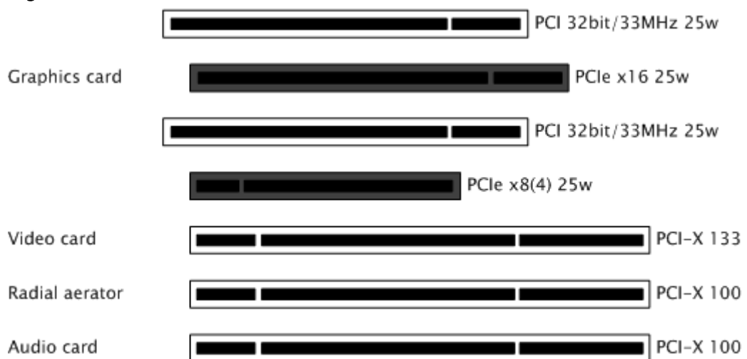
Figure 91: PCI, PCIe and PCI-X slots, HP xw8200
