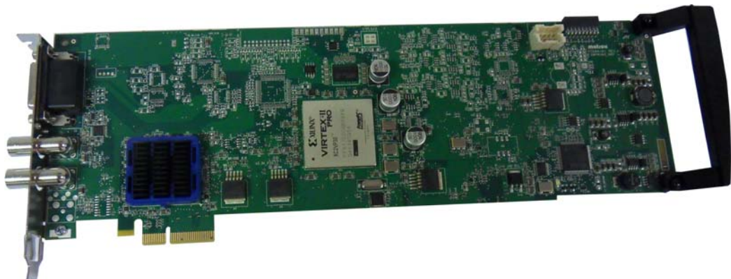
Figure 99: Matrox DSX LE2 card
