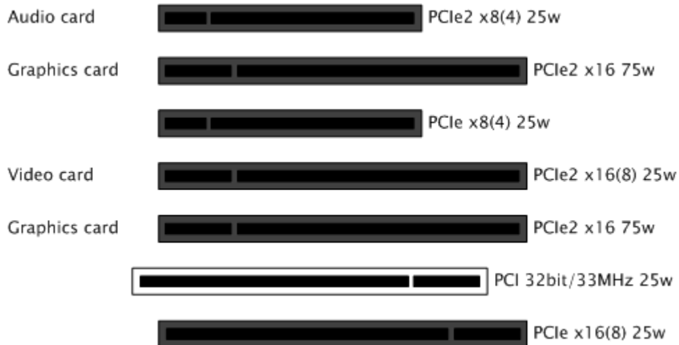
Figure 86: PCI and PCIe slots, HP z800
