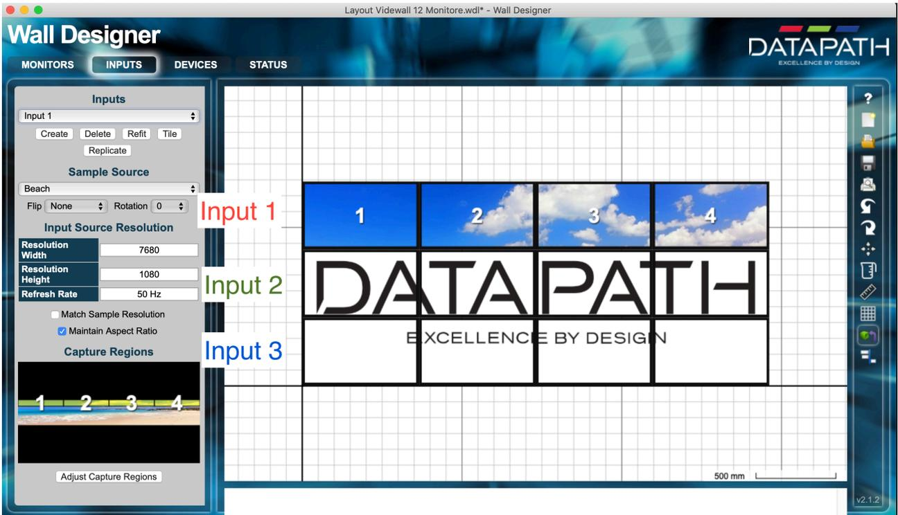
Press **Adjust Capture Regions** if you need to adjust the area the input captured by the various monitors. The alignment of monitors can be fine tuned pixel accurate. Any bezel correction needs also be done here. Make sure the displays align correctly to the configured input.
