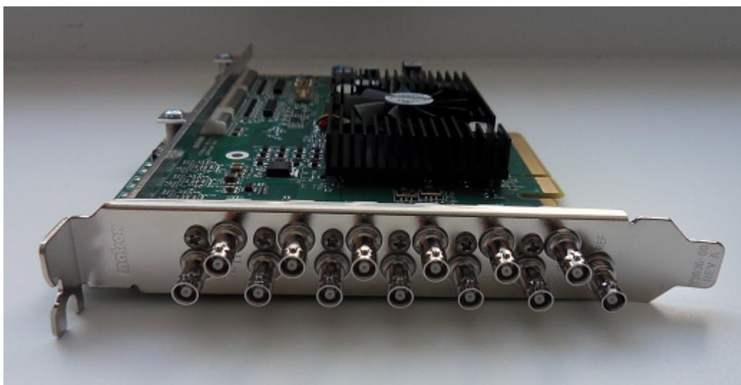
The X.mio3 connectors are labeled 1 through 12 (plus one connector for sync), eight connectors for the LP (low profile) card. As explained, the connectors can be configured for in or out and with various capabilities for clip playback depending on class - with possibilities for firmware class upgrades.
