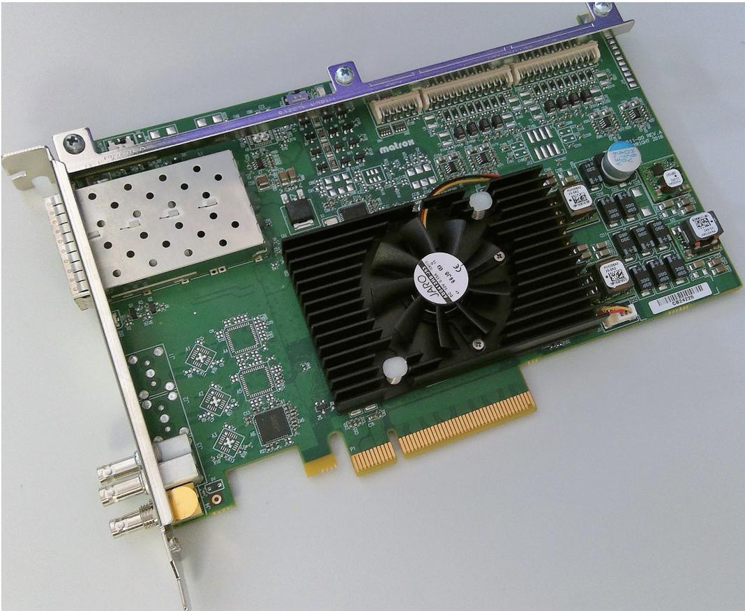
There is one Mini-BNC connector used to connect the card to the house genlock signal. The other two connectors are not implemented.
