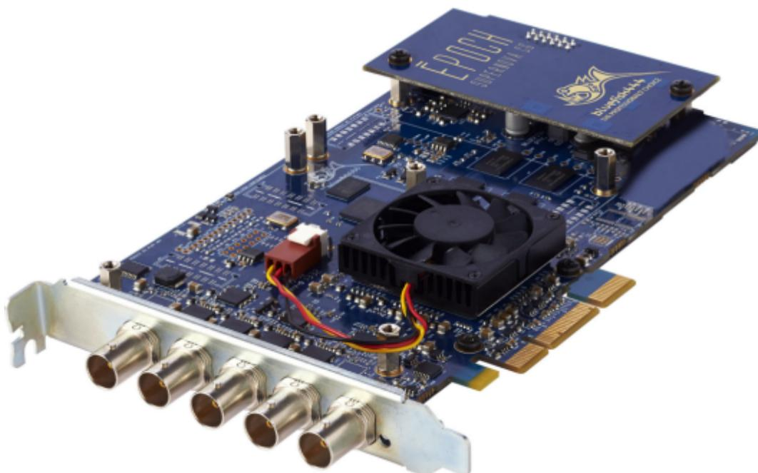
The Epoch | Supernova CG is a 2/3-length PCIe card with bi-directional multi-format I/O BNC connectors that support a number of configurations, up to two dual link channels or four single link channels. For use with Viz Engine, the card needs to be configured with two inputs and two
