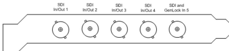
On the Epoch | Supernova CG, the default connector configuration for the five connectors are:
