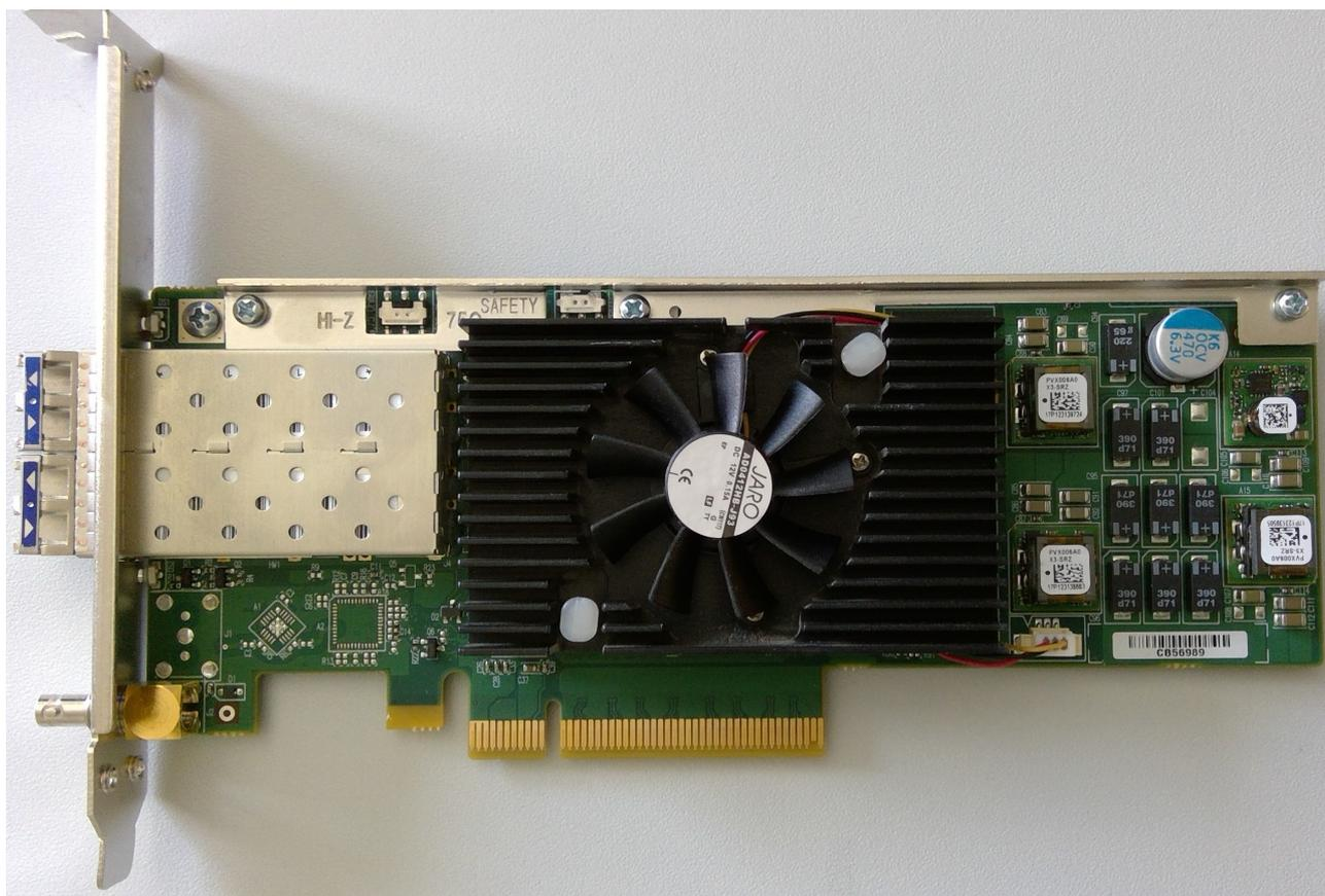
The card contains two enhanced small form-factor pluggable (SFP+) slots, or "bays". In the lower bay is **SFP A**, and hosts input and output channels 1 through 4. The upper bay houses **SFP B**, which hosts all of the redundant channels used with SMPTE ST 2022-7. The board does not have any SDI inputs or outputs. There is one Mini-BNC connector used to connect the card to the house genlock signal. However, the card can also be locked to a SMPTE ST 2059 conform time signal, sent via the SFPs.
