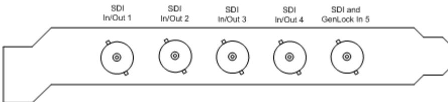
On the Epoch | 4K Supernova, the default connector configuration for the five connectors are:
