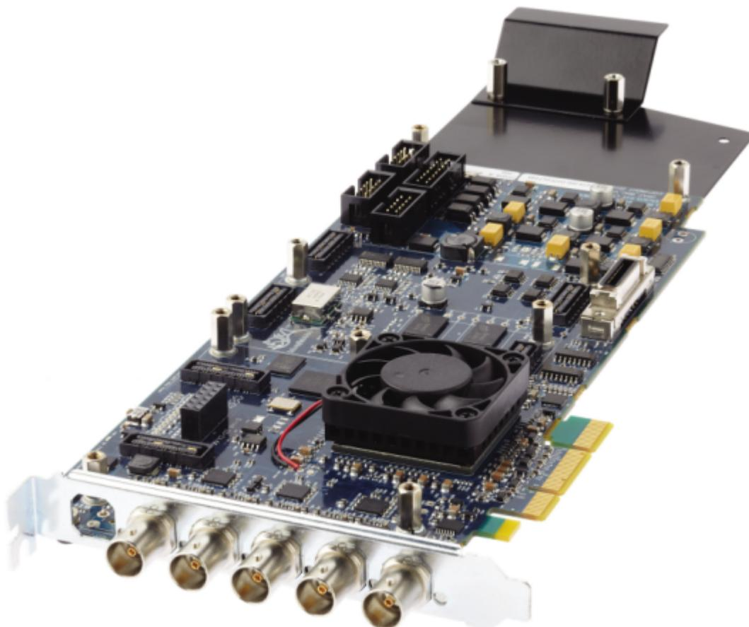
The Epoch | Supernova is a full-length PCIe card with five bi-directional multi-format I/O BNC connectors that support a number of configurations with up to two dual link channels or four single link channels. For use with Viz Engine, the card needs to be configured with two inputs and two outputs.
