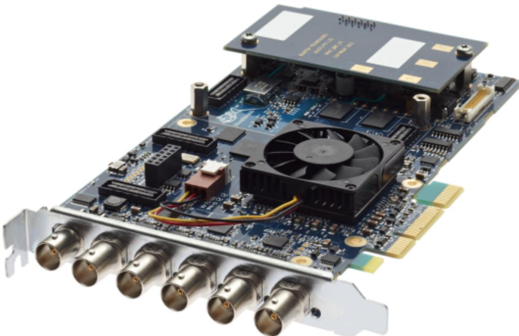
The Epoch | Supernova S+ is a 2/3-length PCIe card with bi-directional multi-format I/O BNC connectors that support a number of configurations, up to two dual link channels or four single link channels. For use with Viz Engine, the card needs to be configured with two inputs and two outputs. With six BNC connectors, each of the first four do SD, HD, 3G, ASI, AES and LTC as either input or output. The fifth is the designated GenLock or SD, HD, 3G, ASI or AES (no LTC).
