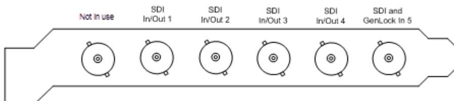
On the Epoch | 4K Supernova S+, the default connector configuration for the six connectors are:
