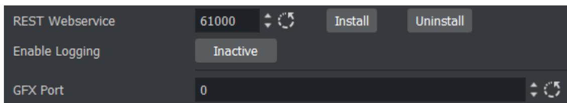
If **User Account Control** is active, press **Install** after setting the Port. The default port for the Viz Engine web service is `61000`. After restarting Viz, the REST interface can be accessed by navigating a web browser to `http://localhost:61000`. The landing page displays the status of the Engine, with information on which mode it is running in and its version number.
