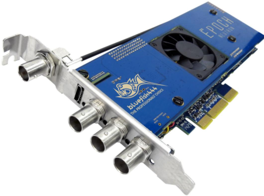
The Epoch | Neutron is a full-length PCIe card with three bi-directional multi-format I/O BNC connectors that support dual link configurations. For use with Viz Engine, the card needs to be configured with one input and one output. Of the three BNC connectors, the first two do SD, HD1.5G, 3G, ASI, AES and LTC as either input or output. The third is used for Genlock.
